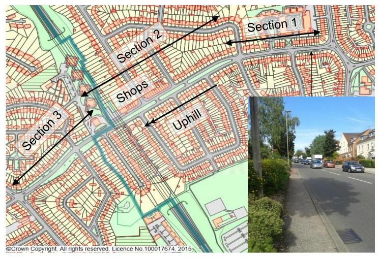
Section 1 - Kerb adjustments needed to accommodate uphill lane but possible high utility diversion costs. Parking restrictions needed.
